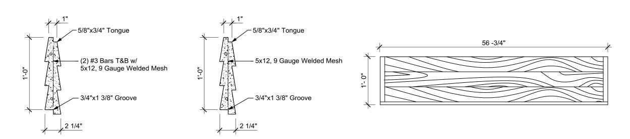
**STANDARD PANEL END PANEL - SECTION MID-WALL PANEL - SECTION**
